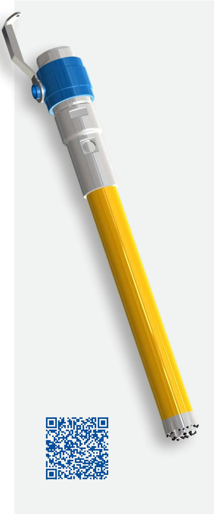
A method of drilling through the overburden with the aid of an outer casing to support the borehole wall is the so-called duplex drilling process. The system depicted here is drilled simultaneously with outer casings and inner rods and driven by a hydraulic drifter. The drill string thus experiences both rotation and percussion.
