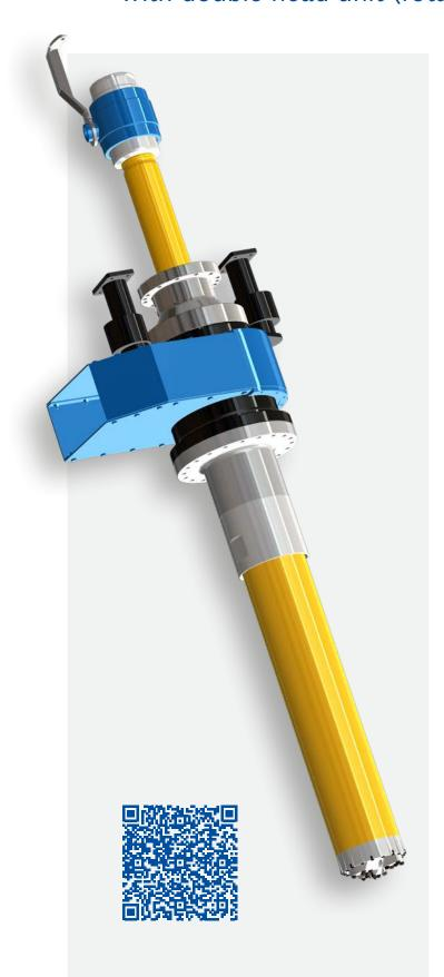
Depending on the intended purpose of the borehole, for instance, to support a bored diaphragm wall, or a subterraneous curtain wall, a cased drilling system is necessary to realise such a borehole. The system listed here features an external and an internal drill string, respectively. The internal drill string is driven by a hydraulic drifter, while the outer drill string is driven by a rotary head or vibro drill head unit, each drill string driven independently from the other.
