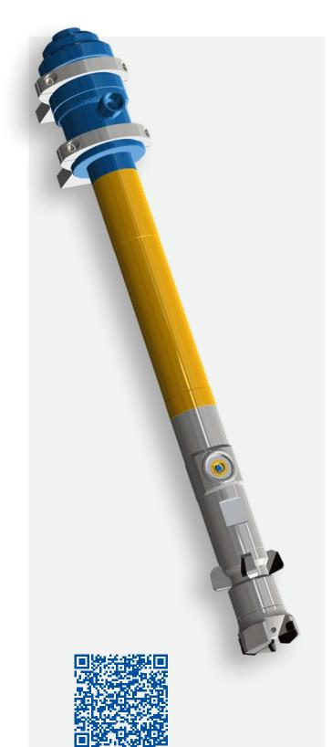
This drilling system is an erosion based system that creates in situ engineered geometries, such as columns, of mixed soil-cement in the subsoil. The aim is to improve the ground conditions by i. e. consolidation, vertical shoring or slicing the soil structure by means of a high velocity jet of grout at pressures of 100 bar (1450 psi) to 600 bar (8700 psi). The drill tools have been specifically designed to withstand these high pressures.
