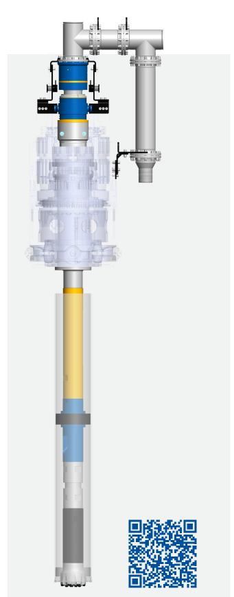
Reverse Circulation (RC) drilling is a drilling method, mostly associated with mining and exploration, where it is used to quickly and economically obtain mineral uncontaminated samples from the ground.
